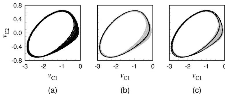
FIG. 4. Measured phase space projections of the double scroll oscillator in the (a) uncontrolled state, (b) controlled period-1 UPO, and (c) controlled period-2 UPO.
