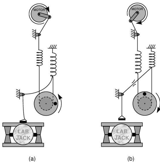
FIG. 1. Configuration of the chaotic driven pendulum, including the mechanical limiter in the (a) slack and (b) taut positions.
