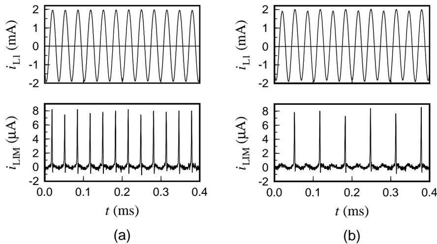
FIG. 5. Control current  $i_{LIM}$  and tank current  $i_{L1}$  compared for stabilized (a) period-1 and (b) period-2 UPOs of the double scroll circuit.
