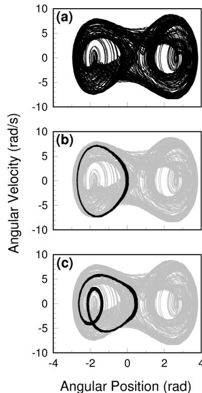
FIG. 2. Measured phase space projections for the pendulum in the (a) uncontrolled state, (b) controlled period-1 UPO, and (c) controlled period-2 UPO.
