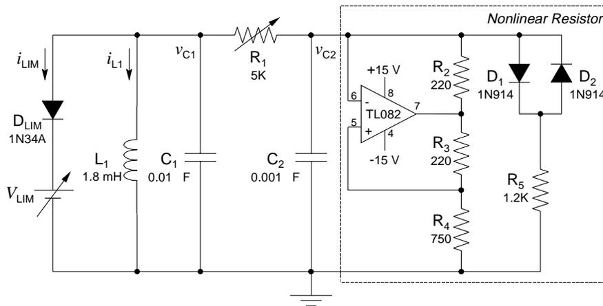
FIG. 3. Double scroll circuit including the diode limiter  $D_{LIM}$  and control level adjustment  $V_{LIM}$ .
