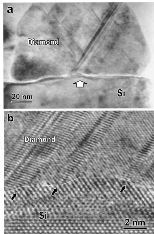
FIG. 2. (a) A low magnification [110] image of a diamond grain. An arrow shows a hillock at the central part of the interface. The majority of twins occur near the hillock. (b) Enlargement of the hillock area in (a). A dotted line traces the facet morphology of the hillock. Three arrows mark the facet edges on the sides of the hillock, where the {111} lamellae start.
