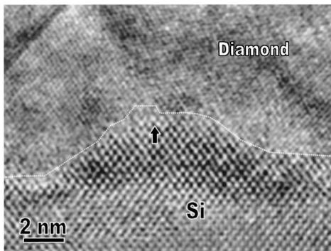
FIG. 3.  $[110]$  lattice image of a diamond grain with a tilt angle of about  $6^\circ$  around the  $[110]$  axis, showing a small  $(001)$  facet on top of the hillock. An arrow denotes a facet edge which induces a twin boundary.
