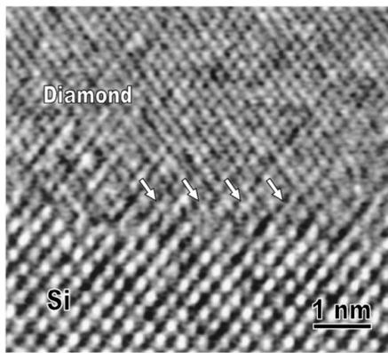
FIG. 1. A lattice image of the interface between diamond and silicon. The micrograph was taken along the [110]-zone axis of diamond and silicon crystals.
