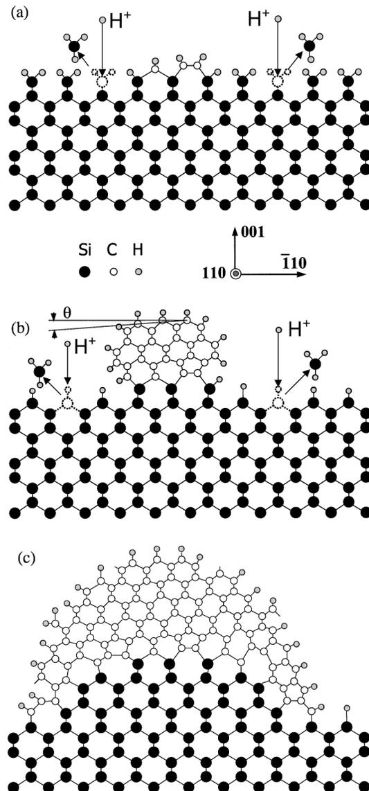
FIG. 4. Schematic sketches illustrating the sequence of formation of the surface hillock and diamond nucleus. (a) The initially deposited carbon configuration and  $\text{H}^+$  ion etching on the silicon  $(001)$  surface, (b) further etching of the silicon surface and formation of tilted diamond nucleus, and (c) further growth of the nucleus and formation of the surface hillock due to etching.
