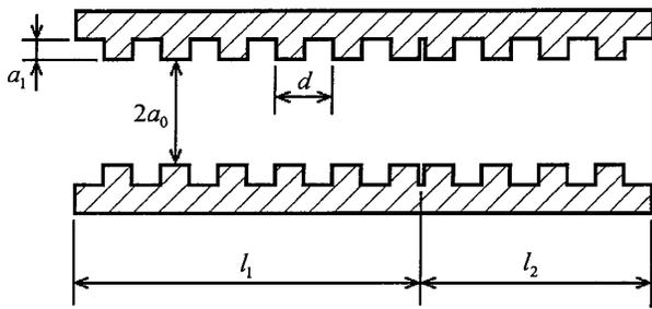
FIG. 1. Scheme of Bragg resonator with step of phase of corrugation.
