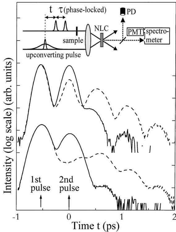
FIG. 1. Inset: Schematic of the experimental setup. NLC stands for nonlinear crystal and PD stands for photodiode. For a time delay  $\tau = 550$  fs equal to the HH-LH beating period, transmitted pulse shapes probed by time-resolved up-conversion are plotted for  $\Delta\phi = \pi$  (solid) and 0 (dashed) when the intensity ratio between two incident pulses ( $I_2/I_1$ ) is 0.59 (upper) and 0.12 (lower).
