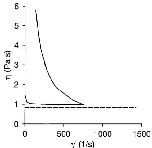
FIG. 2. Apparent viscosity  $\eta$  (Pa s) as a function of strain rate  $\dot{\gamma}$  ( $1/\text{s}$ ) for the flow past a gel of shear modulus 2354 Pa and thickness 4490  $\mu\text{m}$ . The fluid thickness is 300  $\mu\text{m}$ , and the shear rate was increased at the rate of 4 Pa/s. The broken curve shows the result for the same fluid thickness between rigid surfaces.
