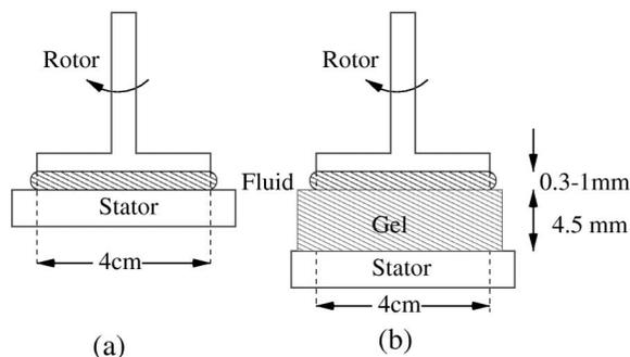
FIG. 1. Rheometer used in the experiments. (a) Unmodified; (b) modified.
