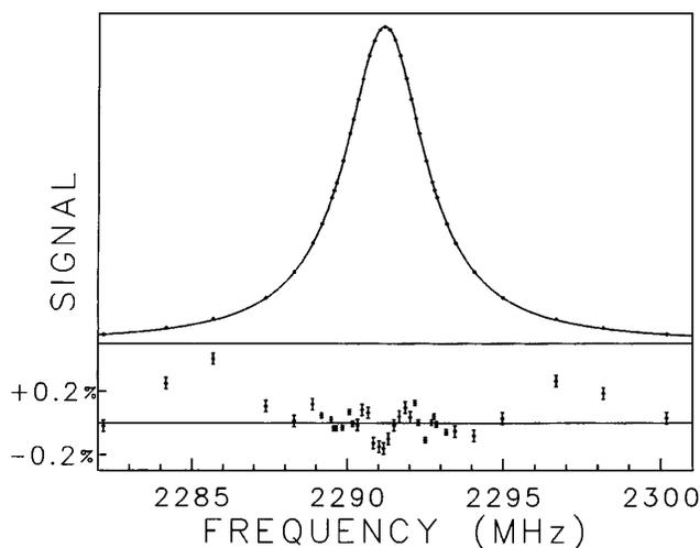
FIG. 2. Averaged data, Lorentzian fit, and residuals. Note the smaller error bars for the points near half maximum, which are repeated 5 times more often than the other points.
