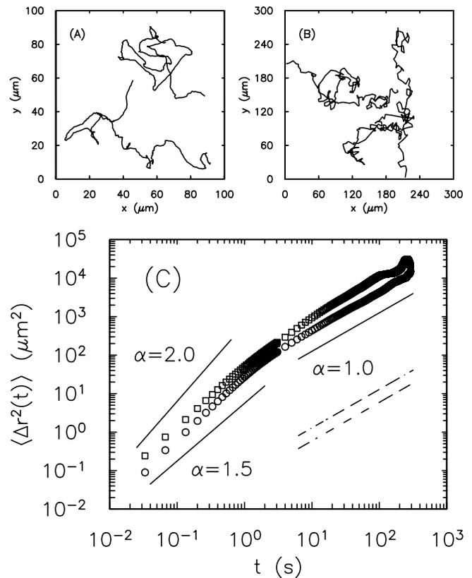
FIG. 2. (A) Motion of two  $10\ \mu\text{m}$  beads followed for 20 s. (B) The same beads followed for 3 min. (C) The MSD measurements of PS beads with diameters  $4.5$  (squares) and  $10\ \mu\text{m}$  (circles) are shown. The bead concentrations were  $\sim 10^{-3}\ \mu\text{m}^{-2}$ . The solid lines with slopes  $\alpha = 2.0$ ,  $1.5$ , and  $1.0$  are guides to the eyes. The two dashed lines correspond to the thermal diffusion of  $4.5$  and  $10\ \mu\text{m}$  particles, respectively.
