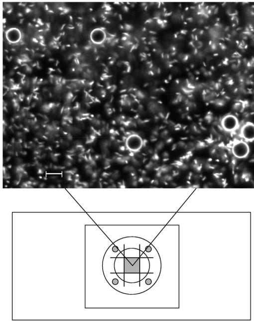
FIG. 1. The experimental setup and the fluorescence image of *E. coli* with  $10\ \mu\text{m}$  PS spheres. The soap film, the square gray area in the figure, was enclosed in an aluminum cell with glass windows. The humidity in the cell was maintained by four water drops as indicated. The scale bar is  $10\ \mu\text{m}$ .
