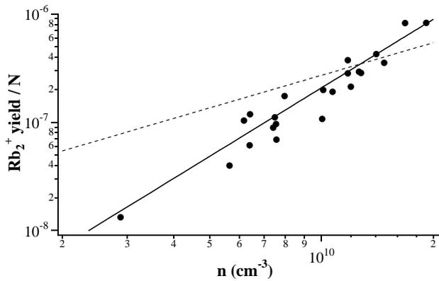
FIG. 4. Number of molecular ions per trapped atom and per pulse as a function of the peak atomic density. The solid curve is the best fitting power function to the data, having an exponent  $2.1 \pm 0.2$ . The dashed line is the best fit for a linear function. The absolute error in the density determination is about 50%, while the relative error is a factor of 2 lower.
