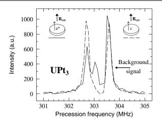
FIG. 1. Two Fourier transforms of spectra recorded at 2.6 K with  $B_{\text{ext}} = 2.3$  T.  $\mathbf{B}_{\text{ext}}$  is parallel to either the  $a^*$  or c axis. The background signal was intentionally enlarged in this measurement to evidence the difference between the applied field and the field at the muon site. This was achieved by fixing a 10-mm-diameter Ag mask on the sample, resulting in a reduced effective sample size. The line at ~303.6 MHz originates from the Ag mask.
