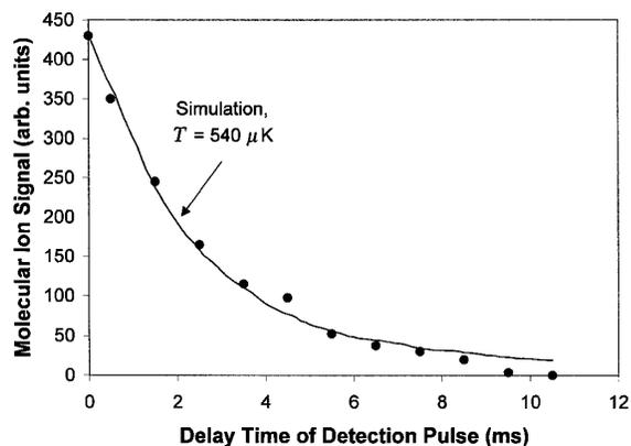
FIG. 4. Decay of the  $K_2^+$  signal after the 853 nm laser is switched off with an acousto-optic modulator. Simulation results depend slightly on the length of the detection region, here taken to be 5 mm, somewhat shorter than estimated by other methods.
