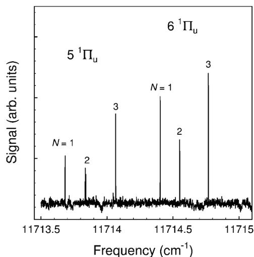
FIG. 2. Scan of the second-step excitation laser at 853 nm, showing transitions from the  $1^1\Pi_g$ ,  $\nu = 89$ ,  $J = 2$  level to rotational levels of  $5^1\Pi_u$ ,  $\nu = 28$  and  $6^1\Pi_u$ ,  $\nu = 13$ .
