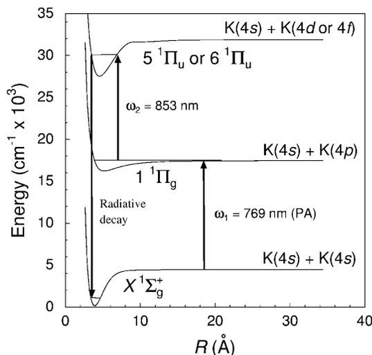
FIG. 1. Formation of ground-state potassium molecules by two-step photoassociation. Potential curves are from Ref. [14]. The second excitation step accomplishes an “ $R$  transfer” to short internuclear distances. The ground state can be populated both by direct radiative decay and cascades through intermediate singlet states.
