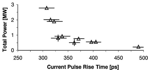
FIG. 3. Power dependence on current pulse rise time.
