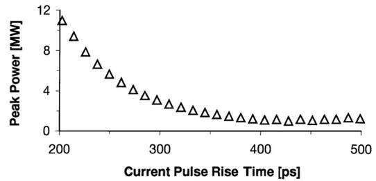
FIG. 4. Simulations of the peak power as a function of current pulse rise time for a parabolic-shaped electron pulse.
