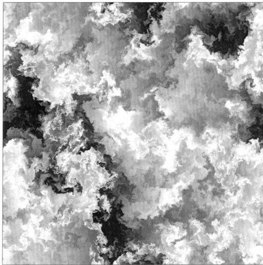
FIG. 1. A snapshot of the scalar fluctuation field for the injection by a mean gradient. Grey scale is coded according to the deviation from the average value (from white to black).
