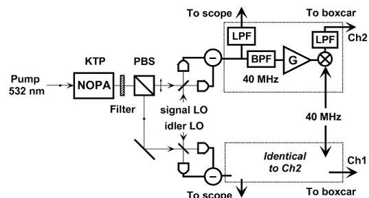
FIG. 1. A schematic of the experimental setup. NOPA, nondegenerate optical parametric amplifier; LOs, local oscillators; PBS, polarizing beam splitter; LPFs, low-pass filters; BPF, bandpass filter; G, electronic amplifier. Electronics in the two channels are identical.
