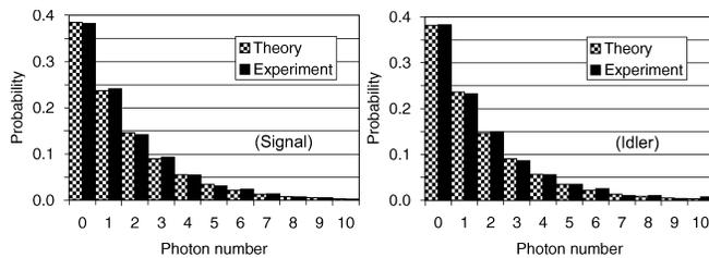
FIG. 3. Marginal distributions for the signal and idler beams reconstructed from the same data as the distribution in Fig. 2(a). Theoretical distributions for the same mean photon numbers are also shown.
