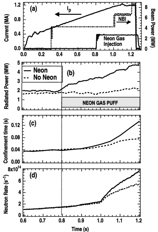
FIG. 1. Discharge parameters for the radiative and reference shots: (a) beam power, plasma current, and neon puff, (b) radiated power, (c) confinement time, (d) neutron rate, showing the relative improvement in performance after the neon puff. Note the different time scales for (a) and (b) through (d).
