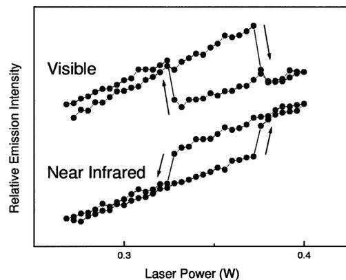
FIG. 2. Power dependence of visible and near-infrared luminescence intensity in a thin sample of  $\text{Yb}^{3+}$  and  $\text{Tm}^{3+}$  doped glass at room temperature. The arrows indicate the directions in which the intensities are changing.
