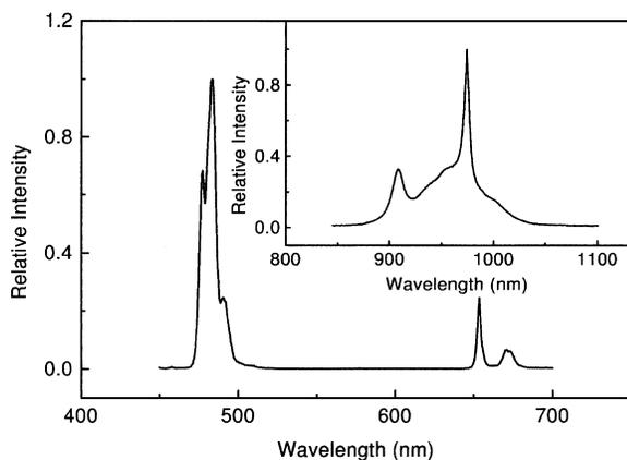
FIG. 1. Unpolarized emission spectra of  $\text{Yb}^{3+}$  and  $\text{Tm}^{3+}$  ions in glass excited at 960 nm. The main figure shows visible emission features. The inset shows near-infrared emission. Vertical axes have been normalized to the most intense spectral peak.
