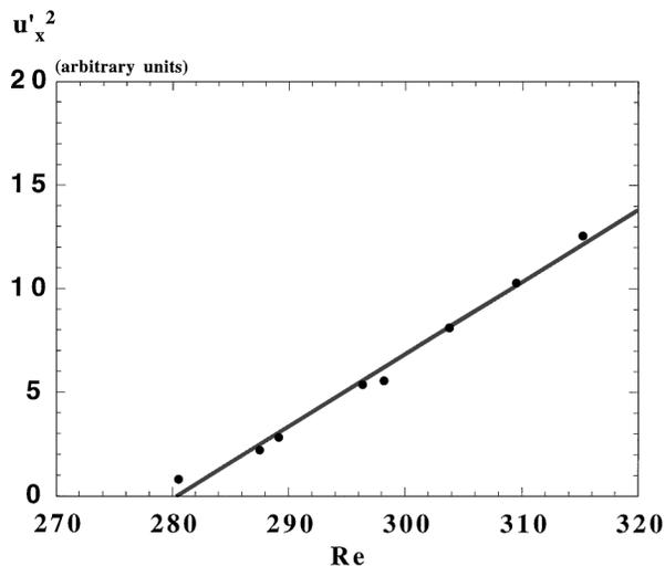
FIG. 4. Energy of the velocity fluctuations  $u'_x{}^2$  versus Reynolds number, measured by LDV.  $x/d = 4.8$ ,  $y/d = -0.2$ ,  $z/d = 0$ .
