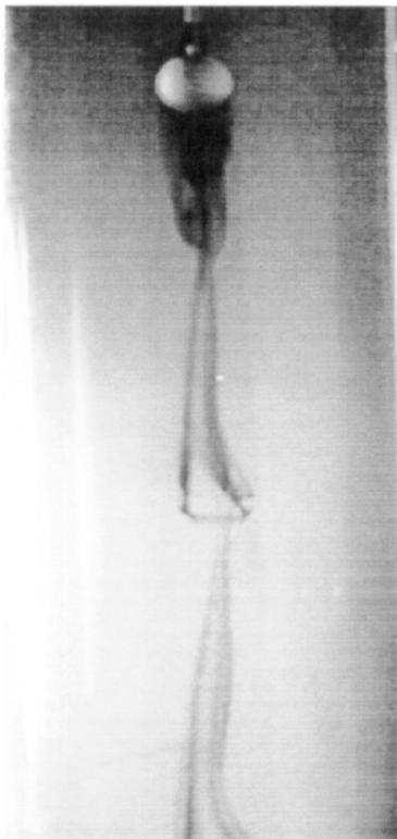
FIG. 2. Periodic vortex shedding obtained by visualization in the water channel, for  $Re = 330$ .
