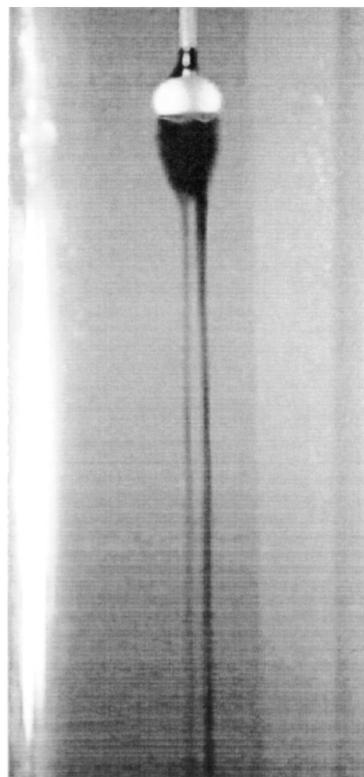
FIG. 1. Two steady trails obtained by visualization in the water channel, for  $Re = 270$ .
