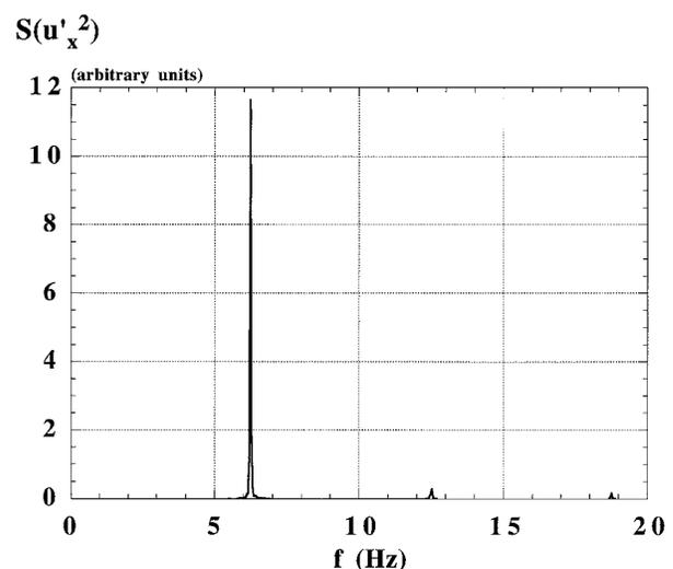
FIG. 3. Spectrum of the streamwise velocity fluctuations  $S_{u_x'^2}$  in periodic regime, measured by LDV.  $Re = 329$ ,  $f = 6.24 \text{ Hz}$ ;  $x/d = 4.8$ ,  $y/d = -0.2$ ,  $z/d = 0$ .
