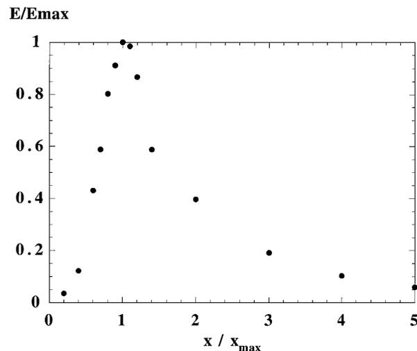
FIG. 6. Variation of the renormalized energy ( $E/E_{\max}$ ) along the flow axis,  $Re = 324$ .
