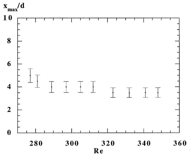
FIG. 7. Variation of the streamwise location of the maximum of energy with the Reynolds number.
