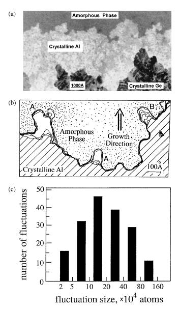
FIG. 1. Results of experiments. (a) An electron micrograph of the crystalline-amorphous interface. The Ge branches are partially seen. (b) Time-resolved characterization of the interface; a sequence of interface lines with intervals of 0.08 sec (every other video frame). Note that this panel is magnified roughly  $10 \times$  compared to part (a). (c) The distribution of avalanche sizes obtained from quantitative measurements of about 200 avalanches.
