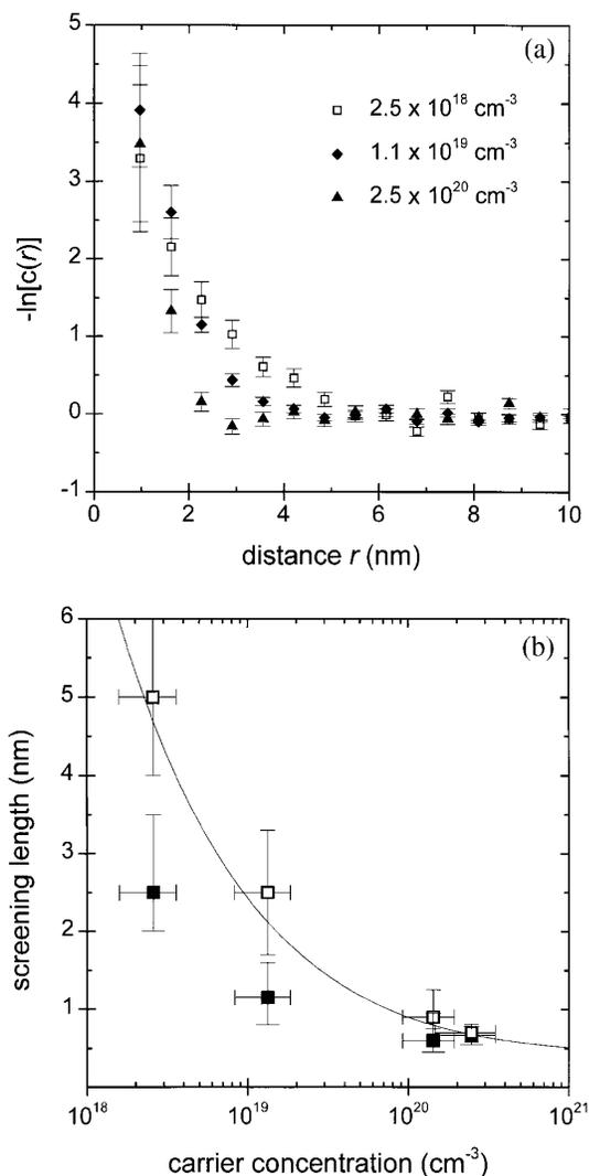
FIG. 2. (a) Negative logarithm of the pair correlation function for three carrier concentrations and (b) values for screening lengths  $R_S$  determined in (a) as a function of the carrier concentration (filled squares). The solid line represents the theoretical screening length calculated according to Eq. (3). The open squares show the screening length corrected for many-body interactions.
