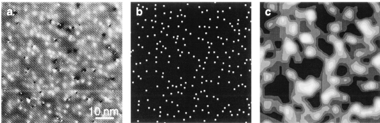
FIG. 1. (a) STM image of a (110) cleavage surface of Zn-doped GaAs acquired at  $-2.4$  V. A long-range contrast variation is superposed onto the atomic-scale corrugation of the atomic rows along the  $[1\bar{1}0]$  direction. The bright and dark contrast features are dopant atoms and vacancies, respectively. (b) Positions of the dopant atoms in (a). (c) Local concentration of the dopant atoms. A high concentration is shown as white contrast. The images show a clustering of the dopant atoms.
