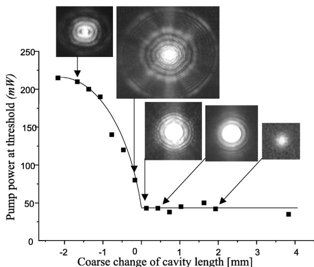
FIG. 2. Pump power threshold as a function of cavity length close to the confocal position, and corresponding signal near field distribution close to threshold.
