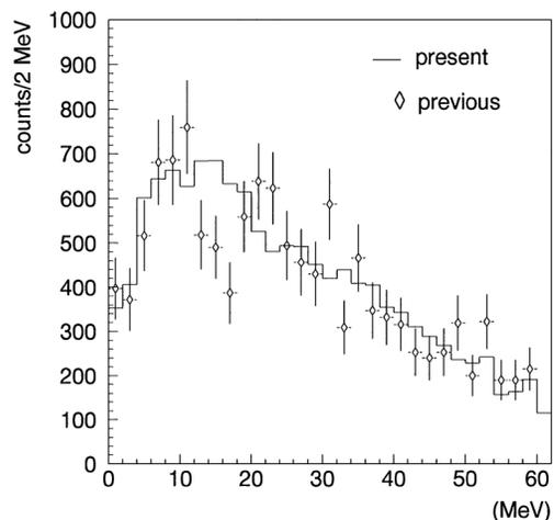
FIG. 2. A direct comparison of the CERN and BNL results for  ${}^9\text{Be}(K^-, \pi^-)$ . The histogram represents the BNL measurement; the CERN data and their error bars were scaled up by about a factor of 10 to allow comparison to the present experiment.
