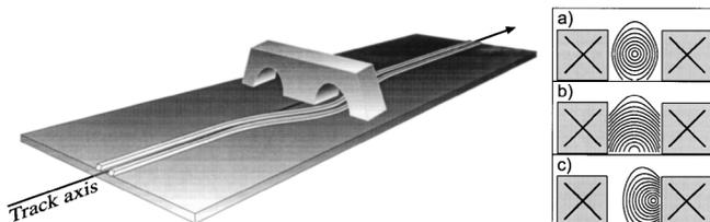
FIG. 2. Detail of magnetic guide. Atoms are guided over a 10-cm distance around three curves each with a 15-cm radius of curvature. A beam block in the middle of the guide blocks the center of the LVIS beam. Insets (a), (b), and (c) show the magnetic field contour lines for no bias, horizontal bias, and vertical bias, respectively.
