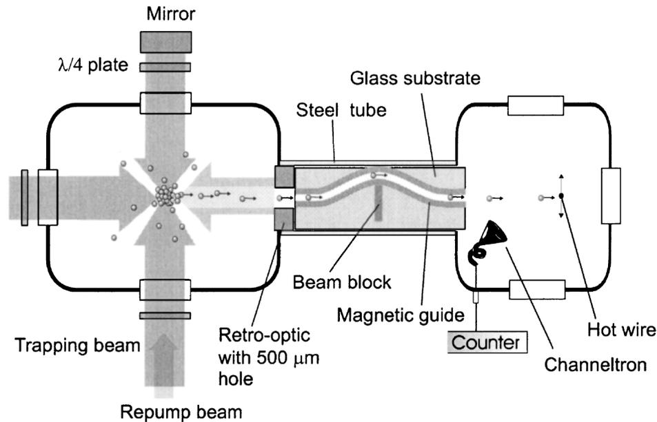
FIG. 1. Schematic of experimental setup. A beam of laser-cooled atoms generated in the source chamber (left) travels toward the magnetic guide between the source and the detection chamber. Atoms enter the tracks and are guided around a barrier. After the guided atoms exit the tracks, they are ionized with a hot wire and ions are counted with a channeltron.
