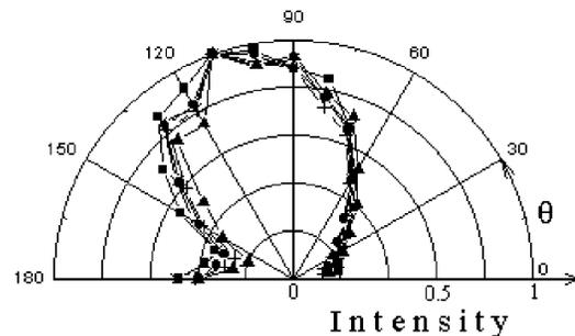
FIG. 5. Polarization dependence of the normalized intensity (with respect to the intensity at  $\theta = 110^\circ$ ) in a PL spectrum of a single InP/GaInP QD, with different symbols for different peaks (Ref. [6]).
