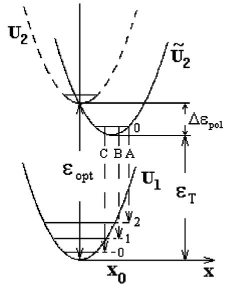
FIG. 2. A schematic plot of various energies which appear in the theoretical model. The transitions A, B, and C give the three corresponding peaks in Fig. 1. See text for details.
