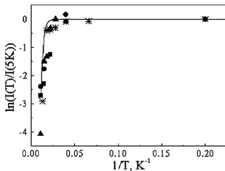
FIG. 4. Temperature dependence of individual peak intensity  $I(T)/I(5\text{ K})$  in a PL spectrum of a single InP/GaInP QD. Different symbols are for different peaks, and the data are collected from more than one QD (Ref. [6]). The solid curve is the theoretical result calculated from Eq. (5).
