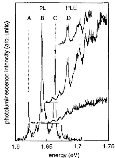
FIG. 1. PL and photoluminescence excitation (PLE) spectrum of a single InP/GaInP QD (from Ref. [1] with permission of the authors).
