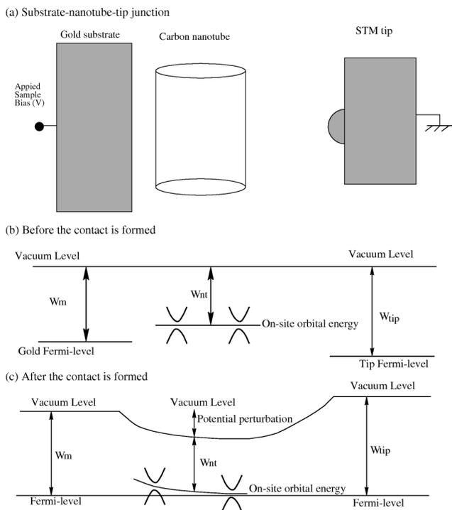
FIG. 1. Illustration of the formation of a substrate-SWNT contact. We show only a semiconducting SWNT here. The work functions of the gold, the SWNT, and the platinum tip are  $W_m = 5.3$  (eV),  $W_{nt} = 4.5$  (eV), and  $W_{tip} = 5.7$  (eV), respectively. (c) shows our picture of the interface Fermi-level positioning.
