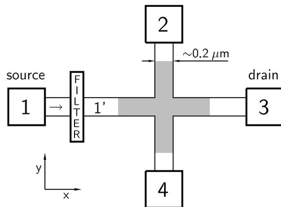
FIG. 1. The cross-junction device. Spin-orbit coupling is supposed to be nonzero in the shadowed area only.
