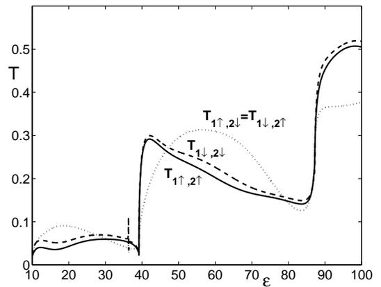
FIG. 2. Energy dependence of the partial transmission coefficients  $T_{1\uparrow,2\uparrow}$ ,  $T_{1\downarrow,2\downarrow}$ ,  $T_{1\uparrow,2\downarrow}$ , and  $T_{1\downarrow,2\uparrow}$  describing transition of polarized electron wave incoming from the lead 1 into the spin-up and spin-down channels of the lead 2.
