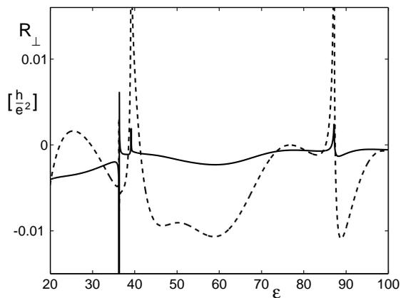
FIG. 4. Hall-like resistance induced by polarization filter transparent for electron waves polarized along the  $\hat{z}$  direction (full line) and along the  $\hat{x}$  direction (dotted line) as a function of the energy.
