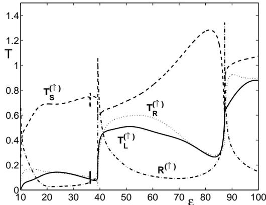
FIG. 3. Scattering coefficients  $T_L^{(\uparrow)}$ ,  $T_S^{(\uparrow)}$ ,  $T_R^{(\uparrow)}$ , and  $R^{(\uparrow)}$  for spin-up polarized electron wave injected from the source (lead 1) as a function of the energy  $\varepsilon$ .
