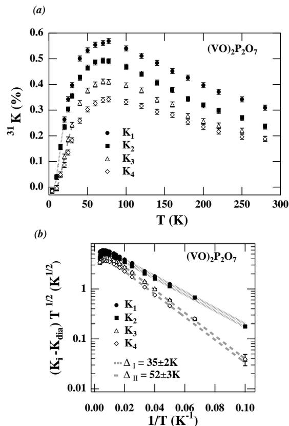
FIG. 4. (a) The temperature dependence of the NMR shifts of the four lines observed in  $^{31}P$  NMR spin-echo spectra. (b) The gap behavior of the four lines. The four lines can be divided into two groups  $K_1, K_2$  and  $K_3, K_4$  from the temperature dependence of the shifts. Both groups show spin-gap behaviors with gap energies of 35 and 52 K, respectively.
