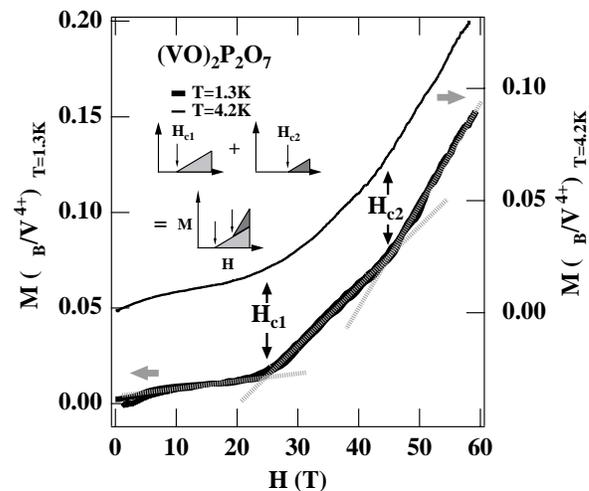
FIG. 2. The field dependence of the magnetization of  $(\text{VO})_2\text{P}_2\text{O}_7$ . The slope of the magnetization curve clearly changes at  $H = 25$  and 45 T as if two independent gap systems coexist in this compound, as schematically shown in the inset.
