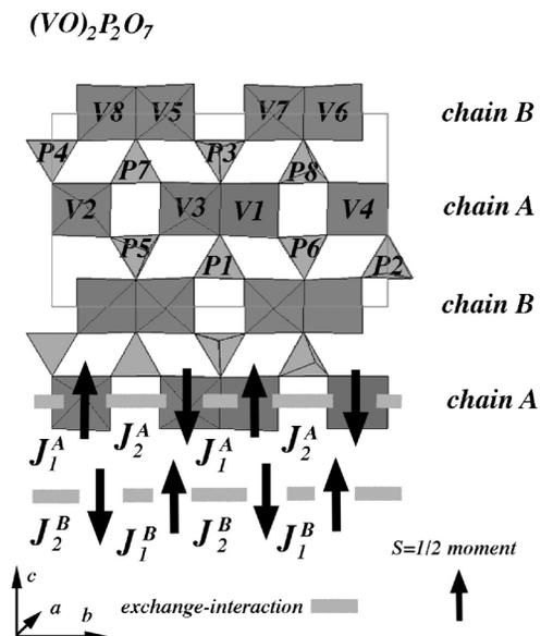
FIG. 1. The crystal structure of  $(VO)_2P_2O_7$ . There exist two kinds of alternating spin chains along the  $b$  axis, chains A and B, in the structure. Both chains consist of the edge-shared  $VO_5$  square pyramids bridged by  $PO_4$  tetrahedra. The schematic view of the magnetic interaction in both chains is also shown.
