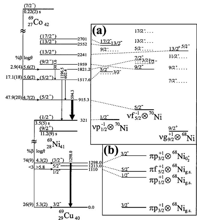
FIG. 2. The experimental decay scheme of  $^{69}\text{Co}$  and  $^{69}\text{Ni}$ , with comparative shell-model calculations for (a)  $^{69}\text{Ni}$  and (b)  $^{69}\text{Cu}$ . Theoretical levels that can be associated with experimental levels are indicated by solid levels and larger fonts. Details are provided in the text.
