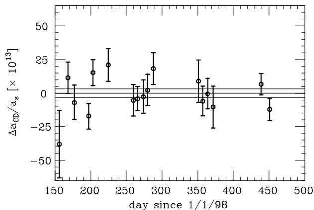
FIG. 4. Each point represents a 4-day measurement of  $\Delta a_{CD}$ . The periods with no points were spent checking for systematic errors or making improvements to the apparatus. The horizontal lines show the  $1\sigma$  statistical plus systematic limits from the combined data.
