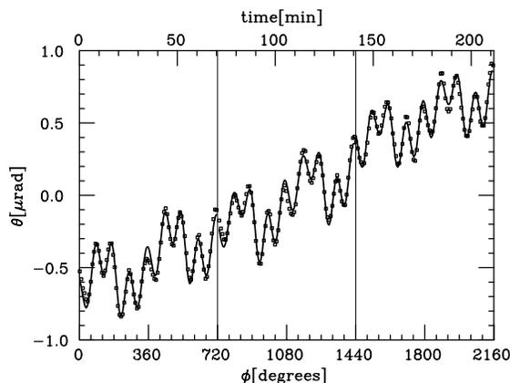
FIG. 2. Sample 2-revolution data segments showing filtered pendulum twist,  $\theta$ , as a function of turntable angle,  $\phi$ . The turntable period equaled 2.5 periods of the free torsional oscillation. Data points were taken at a uniform rate giving 100 points per turntable revolution. The smooth curves show the best fits using Eq. (4).
