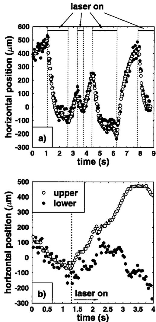
FIG. 5. Analysis of the video sequences in the aligned state at 55 Pa when (a) the upper and (b) the lower particle is pushed by the laser beam.
