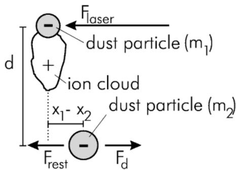
FIG. 6. Interparticle forces in the dust molecule.
