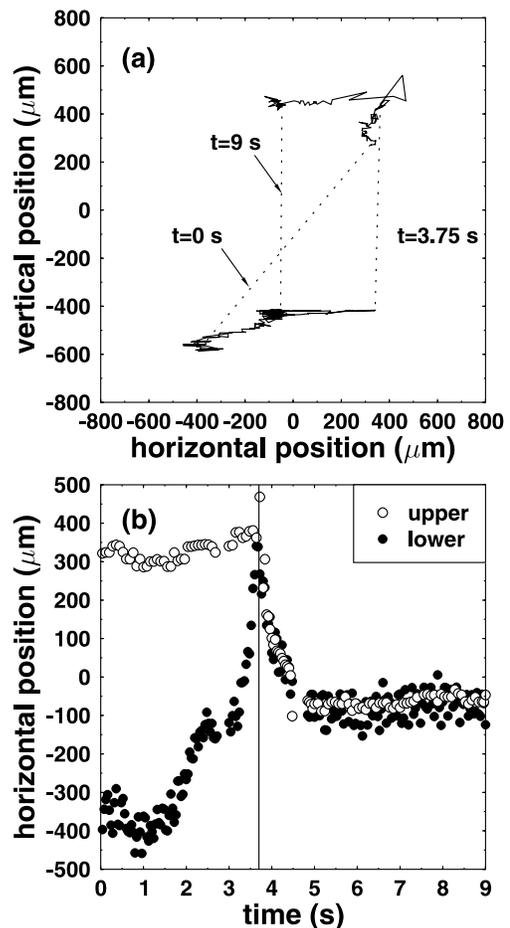
FIG. 3. Analysis of the video sequences during the jump into the aligned state, corresponding to Figs. 2b and 2c. In the upper figure, the particle trajectories as seen by the video camera from the side are shown. The dashed lines connect the particle positions at the given times. The lower figure shows the horizontal positions of the upper and lower particle with time.
