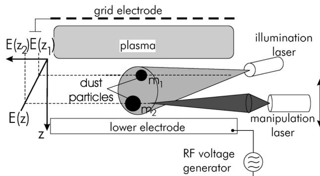
FIG. 1. Scheme of particle trapping in the plasma sheath of an rf discharge. Two particles of different mass find their equilibrium position at different heights above the electrode. Each of the particles can be manipulated by a focused laser beam that allows one to exert a controllable force onto either the upper or the lower particle.
