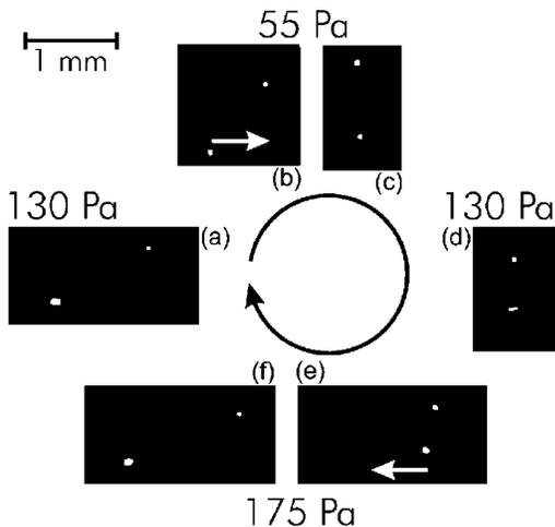
FIG. 2. Behavior of the two trapped particles with change of gas pressure in the discharge between 55 and 170 Pa.
