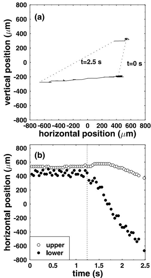
FIG. 4. Analysis of the video sequences during the breakup of the alignment, corresponding to Figs. 2e and 2f. In the upper figure, the particle trajectories as seen by the video camera from the side are shown. The dashed lines connect the particle positions at the given times. The lower figure shows the horizontal positions of the upper and lower particle with time.
