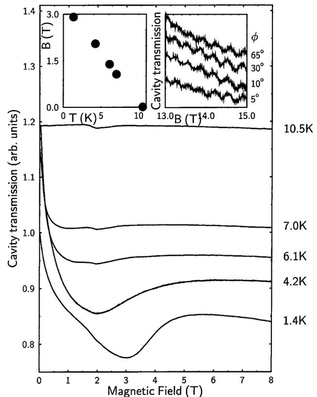
FIG. 2. Main figure: Cavity transmission at fixed  $\phi$  for several temperatures. Left-hand inset: Magnetic field  $B$  of the minimum in transmission versus  $T$ . Right-hand inset: Plot of cavity transmission at  $T = 1.4 \text{ K}$  on an expanded scale showing Shubnikov-de Haas oscillations and their approximate  $\phi$  independence.
