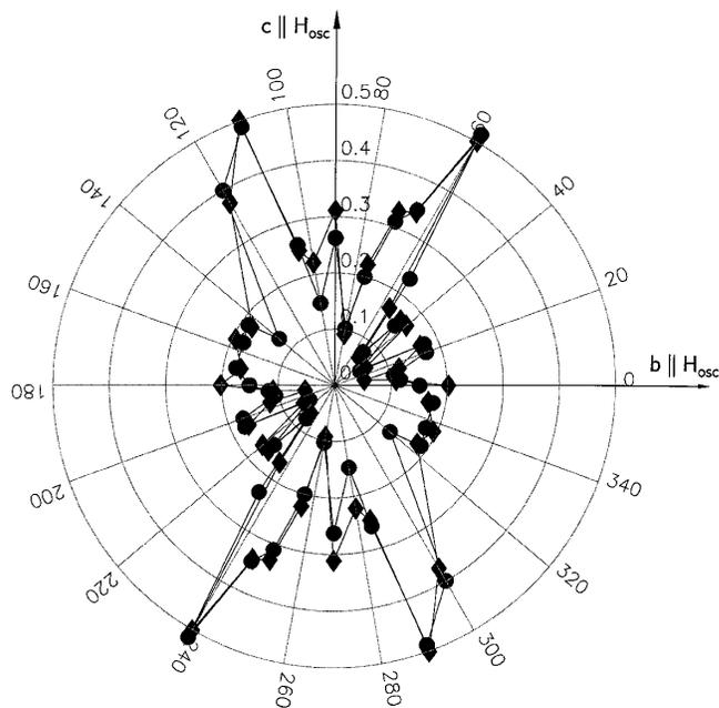
FIG. 3. Normalized amplitude of the minimum in transmission versus azimuthal angle  $\phi$ ;  $\phi = 0$  corresponds to  $\mathbf{H}_{\text{osc}} \parallel \mathbf{b}$  (i.e., induced currents  $\parallel \mathbf{c}$ ) and  $\phi = 90^\circ$  corresponds to  $\mathbf{H}_{\text{osc}} \parallel \mathbf{c}$  (i.e., induced currents  $\parallel \mathbf{b}$ ).
