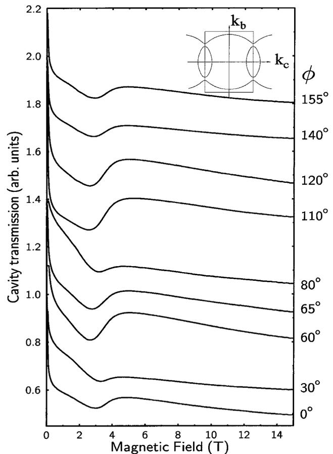
FIG. 1. Main figure: Cavity transmission as a function of magnetic field for several orientations  $\phi$  of the  $\kappa$ -(BEDT-TTF) $_2$ Cu(NCS) $_2$  crystal in the oscillating  $H$  field ( $T = 1.4$  K). Inset: Schematic of the Fermi surface of  $\kappa$ -(BEDT-TTF) $_2$ Cu(NCS) $_2$  (after Refs. [5] and [10]).
