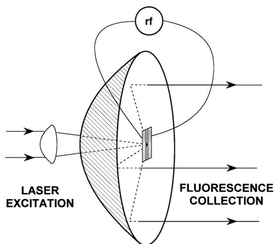
FIG. 1. Schematic diagram of the optical setup used to excite single molecules and to collect their fluorescence. The exciting laser is focused by a lens through a hole in a parabolic collecting mirror onto the sample placed on the front face of the mirror. The Stark shifting rf field is applied via two aluminum electrodes  $18 \mu\text{m}$  apart.
