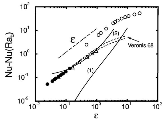
FIG. 1. Log-log plot of  $Nu - Nu(Ra_b)$  vs  $\epsilon$ . Data [5] for  $Ta: 2 \times 10^4$  ( $\bullet$ ),  $3 \times 10^5$  ( $\Delta$ ), and  $5 \times 10^9$  ( $\circ$ ). Numerical calculations [7] (short-dashed curves)  $Ta: 10^4$  (lower curve),  $10^5$  (higher curve).  $\epsilon$  power-law scaling (long-dashed curve). CD scaling (solid curves): (1)  $A = \infty, a = 3.9 \times 10^{-3}, b = 3$ ; (2) fit using  $a = 5.2 \times 10^{-2}, b = 1.15$ .
