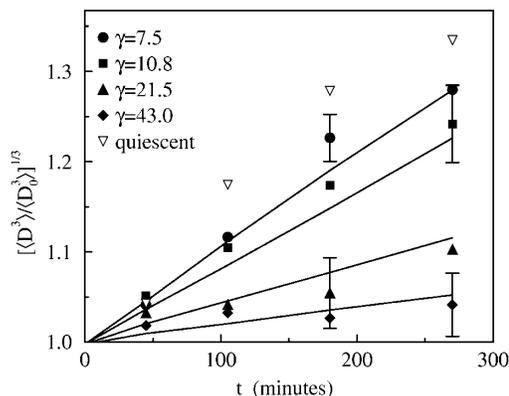
FIG. 2. Variation of the normalized volume average diameter with time for emulsions (1 vol % dispersed phase) subjected to different shear rates ( $\gamma$ ). Points are experimental data and solid lines are the corresponding theoretical predictions using a different fitted value of the coalescence efficiency ( $\epsilon$ ) for each shear rate. The volume average diameter for a standing emulsion is also shown.
