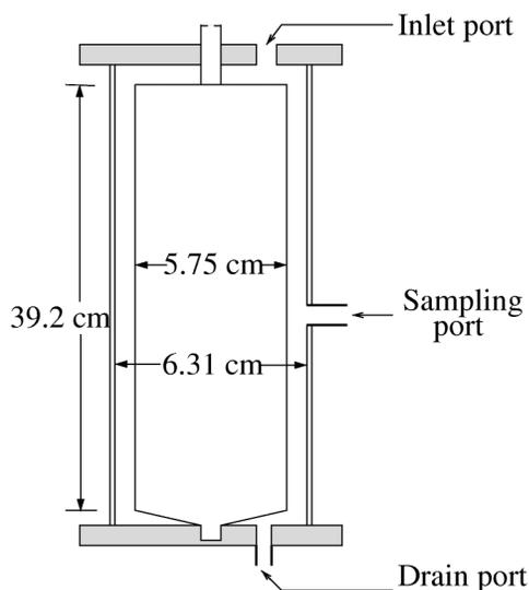
FIG. 1. Schematic diagram of the tangential Couette flow assembly.
