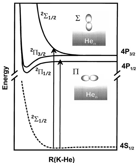
FIG. 3. Schematic potential energy diagram of the K-He complex illustrating different alignments of the excited  $p$  orbital with respect to the helium ( $\Sigma$  and  $\Pi$  states, respectively).
