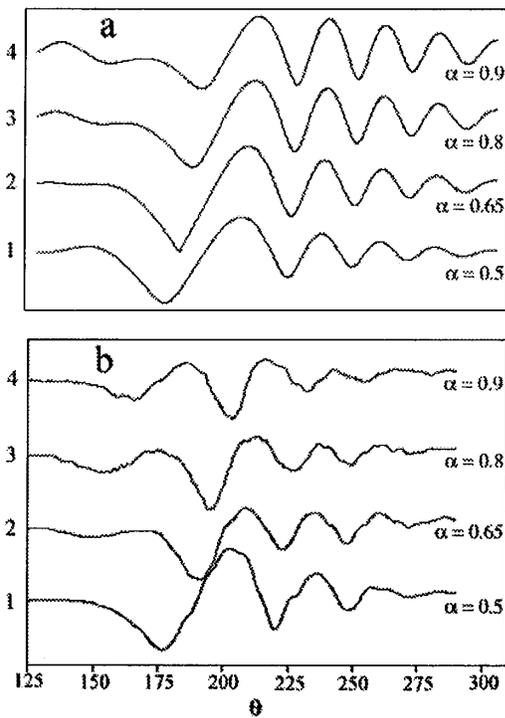
FIG. 4. Experimental surface wave amplitude  $A_s$ , normalized to  $A_0$ , obtained by scanning the water surface around the vortex following a circle of radius  $r = 3$  cm, for  $f = 18$  Hz,  $\lambda = 1.1$  cm,  $c_g = 15.5$  cm/s, and several values of the dislocation parameter  $\alpha$ . Parts (a) and (b) show the theoretical and experimental results, respectively, for comparison.
