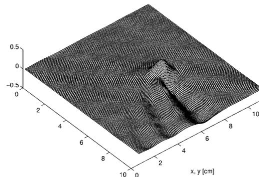
FIG. 3. Experimental surface deflection, obtained by scanning as described in the text, for  $\Gamma \sim 6$  cm<sup>2</sup>/s,  $f = 18$  Hz,  $\lambda = 1.1$  cm, and  $c_g = 15.5$  cm/s. The elevation at the center is the surface deformation associated with the undisturbed vortex.
