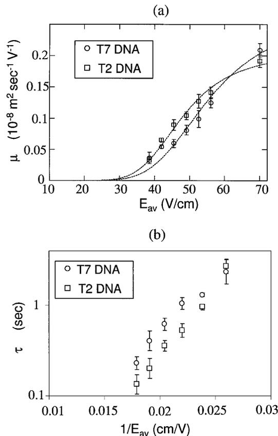
FIG. 5. (a) Mobility of T2 and T7 DNA in a  $4 \mu\text{m}$  period channel with fitting curves.  $t_l = 0.65 \mu\text{m}$  and  $t_s = 90 \text{ nm}$ . (b) Plot of  $\log(\tau)$  vs  $1/E_{av}$ , calculated from (a).
