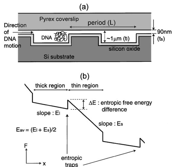
FIG. 1. (a) Schematic diagram of the device. (b) Free energy landscape for DNA in the channel.  $\Delta E$  is the entropic free energy difference between a DNA molecule in a thick region and a thin region.  $E_s$  and  $E_t$  are the electric field in thin and thick regions, respectively.  $E_{av}$  is the average electric field over the channel.
