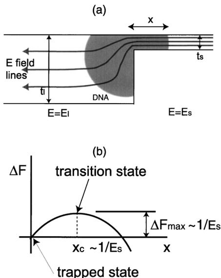
FIG. 4. (a) Escape of a DNA molecule from the trap.  $x$  is the length of DNA section in the thin region. (b) Plot of  $\Delta F$  vs  $x$ . The transition state is when  $x = x_c$ .
