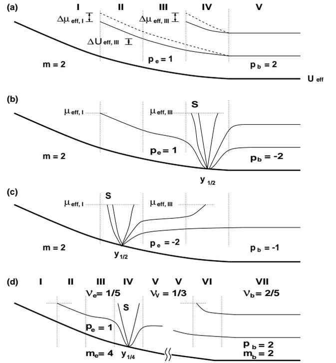
FIG. 2. Schematic diagrams for the CF energy levels (solid lines) for  $m_b = m_e = 2$ ; (a)  $\nu_b = 2/5$ ,  $\nu_e = 1/3$ , (b)  $\nu_b = 2/3$ ,  $\nu_e = 1/3$ , and (c)  $\nu_b = 1$ ,  $\nu_e = 2/3$ . The labeled regions are the same as those in Fig. 1. The heavy lines indicate the effective CF potentials and the dashed lines in (a) represent the energy levels changed by  $\Delta U_{\text{eff}}$ . The energy levels for  $m_b \neq m_e$  are drawn in (d).
