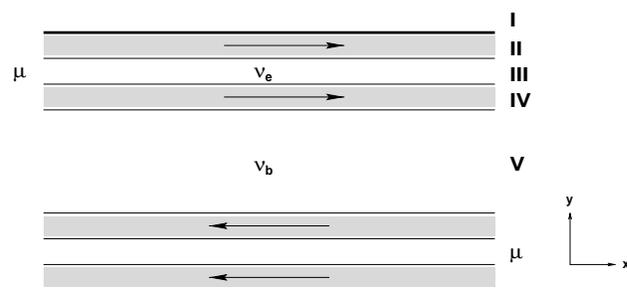
FIG. 1. A schematic diagram for a two-dimensional conductor connected to the left and right reservoirs with the chemical potential  $\mu$ . Compressible (shaded) and incompressible (white) regions are labeled. The arrows indicate additional current flows induced by  $\Delta\mu$ .
