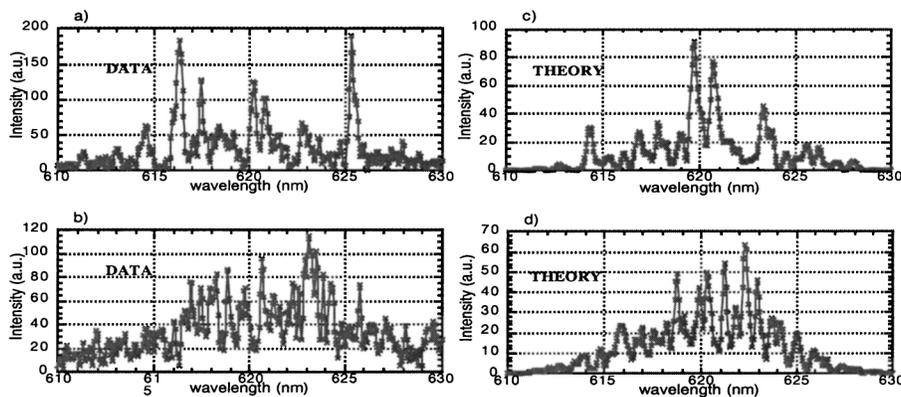
FIG. 2. Comparison of experimental data and simulations. (a) and (b) show typical single shot spectra for a single electron bunch passing through the wiggler for bunch lengths of 1.5 and 4.5 ps, respectively. Numerically generated spectra at the same bunch lengths (c) and (d) reproduce the salient features of the data: level of modulation and characteristic spike width.
