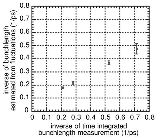
FIG. 4. Reciprocal of the bunch length estimated from fluctuations is compared with time integrated measurements.
