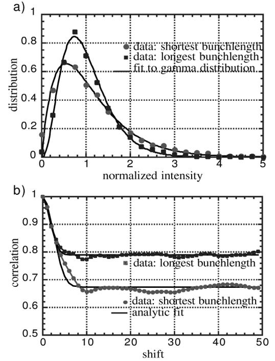
FIG. 3. (a) Measured distribution of intensity fluctuations for shortest (1.5 ps) and longest (4.5 ps) bunch lengths are plotted along with the gamma distribution fit. (b) Average frequency correlation [Eq. (5)] of measured single shot spectra and fit [Eq. (6)] for the shortest and longest bunch lengths.
