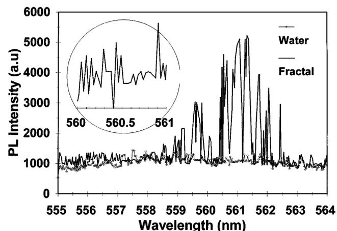
FIG. 2. Luminescence spectrum of  $5 \times 10^{-7}M$  R6G dye solution in microcavity, with [heavy line, neutral density (OD = 5) filters are used] and without (circles, dashed line) fractals, for  $\lambda_L = 514.5\ \text{nm}$ , cw Ar laser excitation. Inset gives detail of spectrum without fractals showing typical mode structure.
