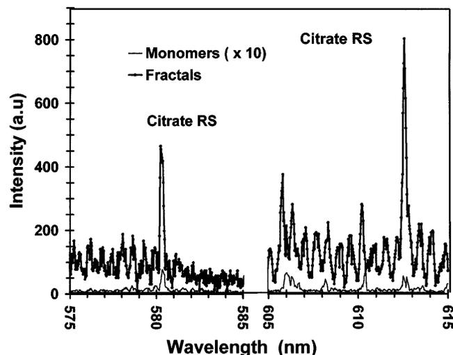
FIG. 4. Inelastic scattering spectra of nonaggregated silver monomers without dye (thin line, lower trace) and fractal aggregated monomers with  $5 \times 10^{-7} M$  dye solution (thick line, upper trace) in microcavity for  $\lambda_L = 543.5$  nm, cw He-Ne laser (maximum power is 0.75 mW).
