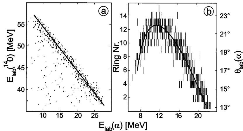
FIG. 1. (a) Energies of coincident  $\alpha$  and  $^{14}\text{O}$  particles. The coplanarity condition has been applied. (b) A two-dimensional scatter plot of  $\alpha$ -particle angle (ring number) vs  $\alpha$  energy for the events from (a), requiring also the correct sum energy. The solid lines represent the expected  $E_{\alpha} - E_{^{14}\text{O}}$  and  $\theta_{\alpha} - E_{\alpha}$  correlations, respectively, for events originating from the midpoint of the target.
