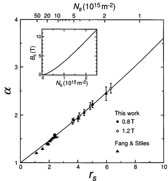
FIG. 3. The enhancement factor  $\alpha = g_{FL} m_{FL} / 0.38 m_e$  vs the strength of the electron-electron interaction. The inset shows the critical magnetic field  $B_c$  calculated using Eq. (1).
