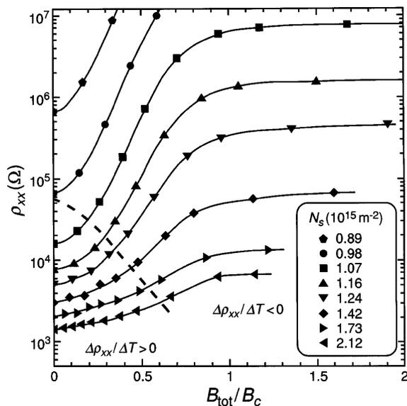
FIG. 4. Resistivity vs  $B_{tot}/B_c$  at  $T = 0.21$  K and  $B_{\perp} = 0$  for various  $N_s$ . The dashed line represents the critical value of  $\rho_{xx}$  at the MIT determined from temperature dependence between 0.21 and 0.91 K.
