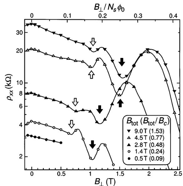
FIG. 5. Diagonal resistivity vs normal component of the magnetic field at  $T = 0.31$  K and  $N_s = 1.46 \times 10^{15} \text{ m}^{-2}$  for several values of  $B_{tot}$ .
