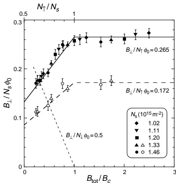
FIG. 6. Positions of the  $\rho_{xx}$  minima for various  $N_s$  are plotted. The solid and dashed lines represent  $B_{\perp}/N_{\uparrow}\phi_0 = 0.265$  and  $B_{\perp}/N_{\uparrow}\phi_0 = 0.172$ , respectively. The dotted line represents  $B_{\perp}/N_{\downarrow}\phi_0 = 0.5$ .
