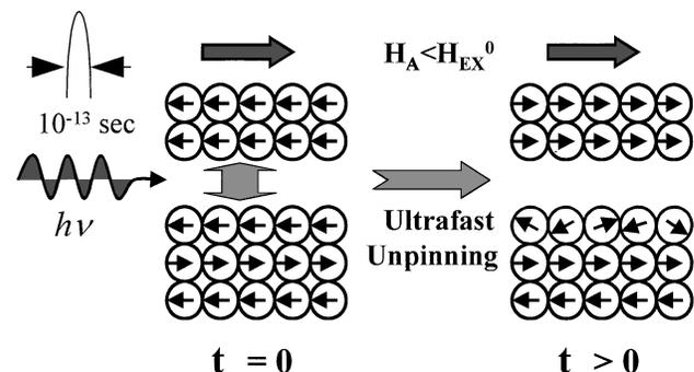
FIG. 1. The concept of optically induced “unpinning” of the exchange bias (field) at FM/AF exchange coupled interface. With the magnetization of the FM layer is initially biased antiparallel to external field, ultrashort pulse photoexcitation triggers a coherent rotation process.
