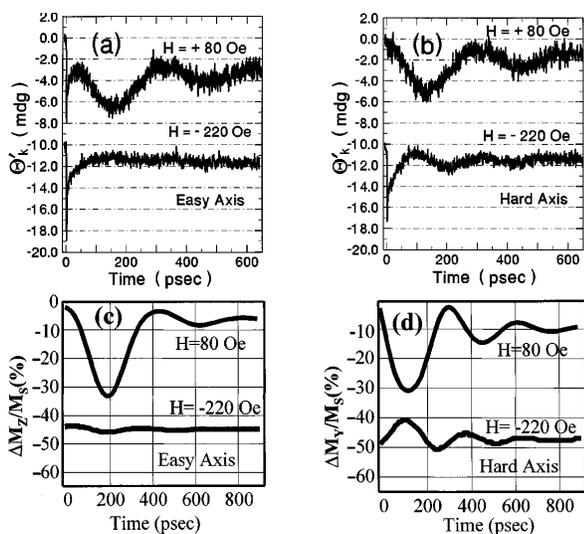
FIG. 3. Time-resolved transient Kerr effect  $\theta'_K(t)$  for the photoexcited NiFe/NiO bilayer in an external field of  $H_A = 80$  Oe, and  $H_A = -220$  Oe. (a) applied along the easy axis, and (b) along the hard axis. Traces (c) and (d) show the results of a model calculation described in the text.
