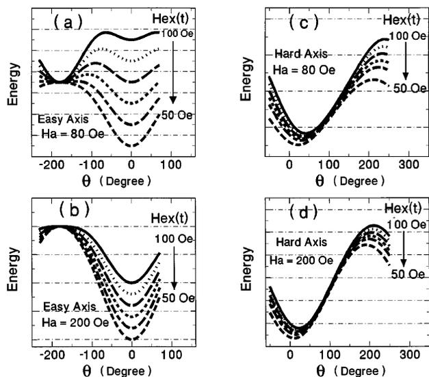
FIG. 4. Energy diagrams for the bilayer system with the exchange bias field  $H_{ex}(t)$  modulated between 100 and 50 Oe. The external field of  $H_A = 80$  Oe and  $H_A = 200$  Oe is applied along the easy axis in (a) and (b), and along the hard axis in (c) and (d).
