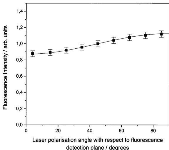
FIG. 3. Dependence of the fluorescence from Na( $3p$ ) on the polarization direction  $\beta$ , with respect to the fluorescence detection plane, of the laser light used to excite the sodium atoms. The full line is a fit to the experimental data:  $1 - 0.13 \cos(2\beta)$ .
