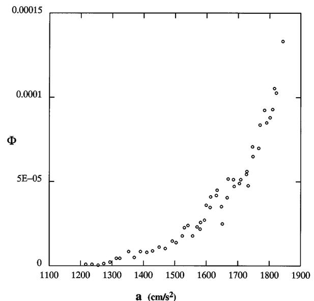
FIG. 2. Droplet rate data from  $\nu = 5$  cS Silicone Oil at 45 Hz: Each point represents the number of droplets (scaled with measurement parameters) produced in a 300 s period.
