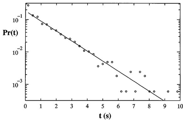
FIG. 4. A histogram of the times between ejections indicates that the distribution is a Poisson distribution and supports a hypothesis that the ejections are independent events.
