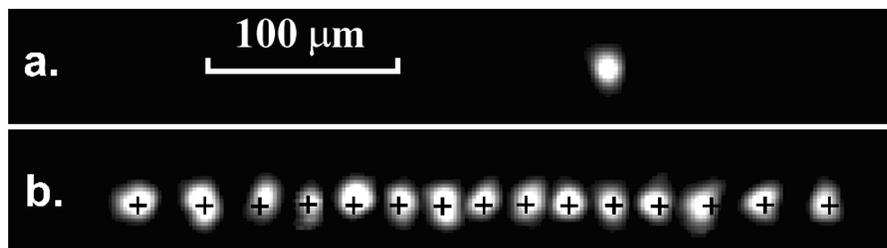
FIG. 2. (a) A single video frame showing the lone  $^{24}\text{Mg}^+$  ion in one of the fifteen sites. (b) The overall structure of the crystal visualized by making a superposition of 15 images in each of which a different site is occupied. The superimposed crosses indicate the positions predicted by molecular dynamics simulations for a string containing 15 singly charged ions.
