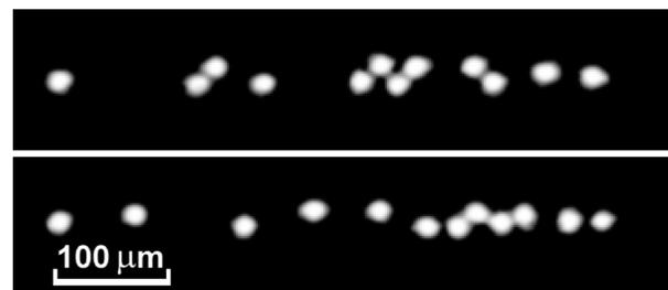
FIG. 4. A sequence of images recorded using only one cooling laser tuned to  $^{24}\text{Mg}^+$ . The images are taken while the ions are migrating due to power imbalance between the two counterpropagating laser beams.
