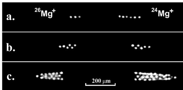
FIG. 3. Three successive images taken during a loading sequence. The  $^{24}\text{Mg}^+$  ions are pushed to the right and  $^{26}\text{Mg}^+$  ions to the left by their respective near resonant cooling lasers. The central region contains sympathetically cooled ions. Note the nearest neighbor separation between ions is ca.  $20\ \mu\text{m}$  while the space between the two magnesium isotopes is ca.  $500\ \mu\text{m}$  wide.
