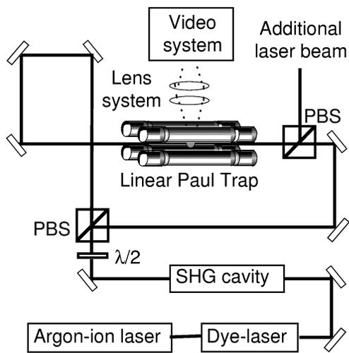
FIG. 1. Schematic overview of the experimental setup. The optional second UV laser beam of a separately adjustable frequency, produced by a similar laser and frequency doubling system, is also shown. PBS (polarizing beam splitter);  $\lambda/2$  (half-wave plate).
