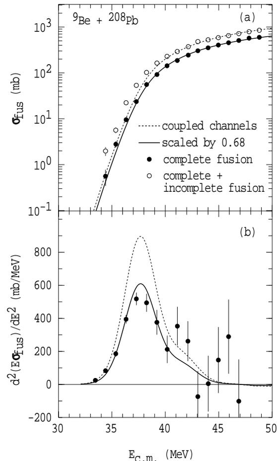
FIG. 2. (a) The excitation function for complete fusion (filled circles) and (b) the barrier distribution for the reaction  ${}^9\text{Be} + {}^{208}\text{Pb}$ . The dashed line is the result of a coupled channels calculation (see text) which ignores breakup effects. The full line is the same calculation scaled by 0.68. The sum of measured complete and incomplete fusion cross sections is given by the hollow circles.
