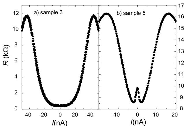
FIG. 2. Resistance vs current for two samples showing different behavior: (a) sample 3 with  $R_T = 3.7$  k $\Omega$  and  $R_s = 11$  k $\Omega$ ; (b) sample 5 with  $R_T = 12.4$  k $\Omega$  and  $R_s = 22$  k $\Omega$ .
