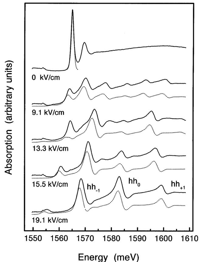
FIG. 1. Solid lines: Experimental absorption spectra of a 67/17 angstrom superlattice for various fields. Dashed lines: Theoretically calculated spectra.
