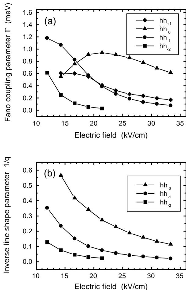
FIG. 2. (a) Fano coupling parameter  $\Gamma$  vs field for various WSL indices  $n$ . (b) Inverse of the Fano line shape parameter  $q$  as a function of field.
