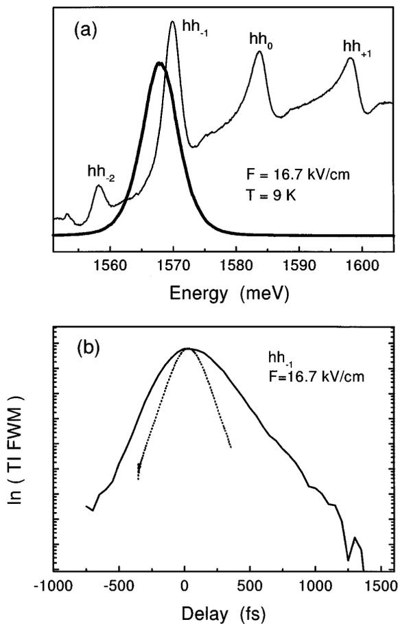
FIG. 3. (a) Example of the excitation conditions for the time-resolved experiments: The laser maximum is shifted approximately 2 meV below the absorption peak (fat line: laser spectrum). (b) Resulting FWM signal in comparison to the autocorrelation of the laser pulse (dashed line).
