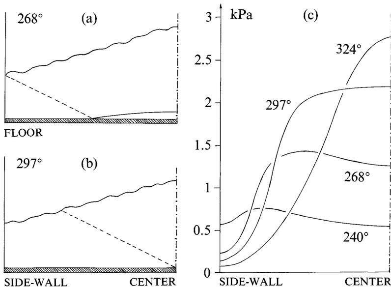
FIG. 2. Status of center-high vibrated bed at phase angles during gap closure. (See Fig. 1 caption for bed description and vibration parameters.) (a) and (b) Show bed profiles at two phase angles: gap closed halfway to center and gap just closed at center, respectively. Dashed lines indicate positions of compaction front. (c) Gives approximate floor pressure profiles at designated phase angles.
