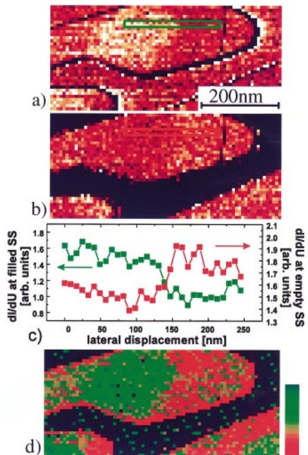
FIG. 3(color). Detail from the data set shown in Fig. 2. (a) In the  $dI/dU$  image measured at  $U = -0.2$  V the left part of the island is brighter than the right part indicating a parallel alignment of the filled surface state spin part with the tip spin polarization at the Fermi level. (b)  $dI/dU$  image measured at  $U = +0.45$  V. (c) Plot of the  $dI/dU$  signal drawn along the line sections indicated above. (d) Asymmetry image (linear scale bar: 23%) calculated from (a) and (b).
