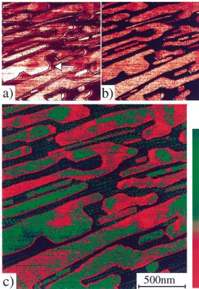
FIG. 2(color).  $dI/dU$  image at the majority [(a)  $U = -0.2$  V] and the minority [(b)  $U = +0.45$  V] surface state peak position. While a strong contrast within the Gd island can be recognized in (a), a weaker and opposite contrast is present in (b). The arrow indicates where an accidental tip change occurred. (c) In the asymmetry image (linear scale bar: 23%) the contrast is enhanced and tip changes less visible.
