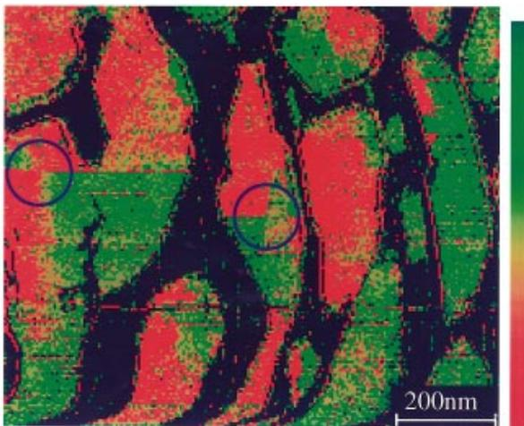
FIG. 4(color). Asymmetry image (linear scale bar: 19%) of a Gd sample measured with a 100–200 ML thick Fe coating on the tip. The blue circles indicate two Gd islands whose magnetization were accidentally switched probably due to interaction between tip and sample mediated via the stray field.
