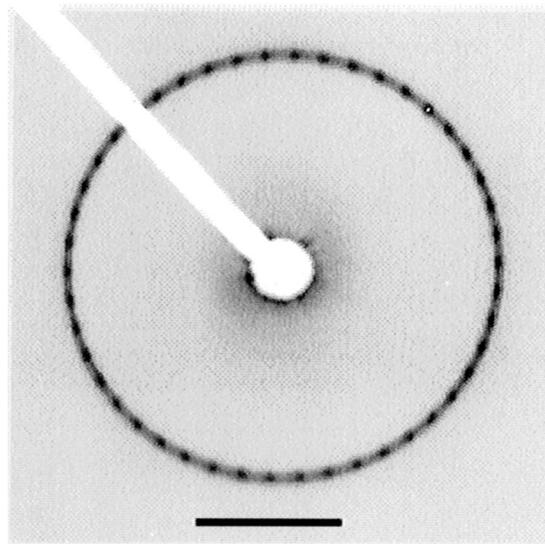
FIG. 2. X-ray diffraction pattern of the TGB<sub>A</sub> phase upon heating at  $T = 101.4 \text{ }^\circ\text{C}$ . This pattern exhibits 46 spots equispaced along a ring and is the signature of a commensurate TGB<sub>A</sub> phase. The line indicates the buffing direction.
