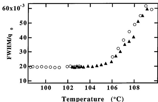
FIG. 4. Variation of the ratio  $\text{FWHM}/q_0$  as a function of temperature (circles: upon cooling; full triangles: upon heating). FWHM is the width (full width at half maxima) of the homogeneous diffuse ring and  $q_0$  the scattering vector at maximum intensity. The width remains constant in the presumed  $N_L^*$  phase and increases in the cholesteric phase.
