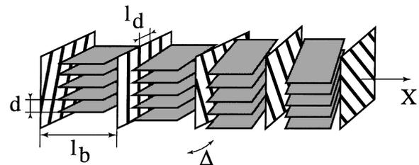
FIG. 1. Schematic representation of the  $TGB_A$  phase (twist grain boundary). The pitch axis is along the  $x$  direction. Blocks of SmA layers of spacing  $d$  are separated by regularly spaced twist grain boundaries separated by a distance  $l_b$ . The distance between screw dislocations within a grain boundary is  $l_d$ .
